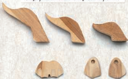
Roughly cut & sanded feet
